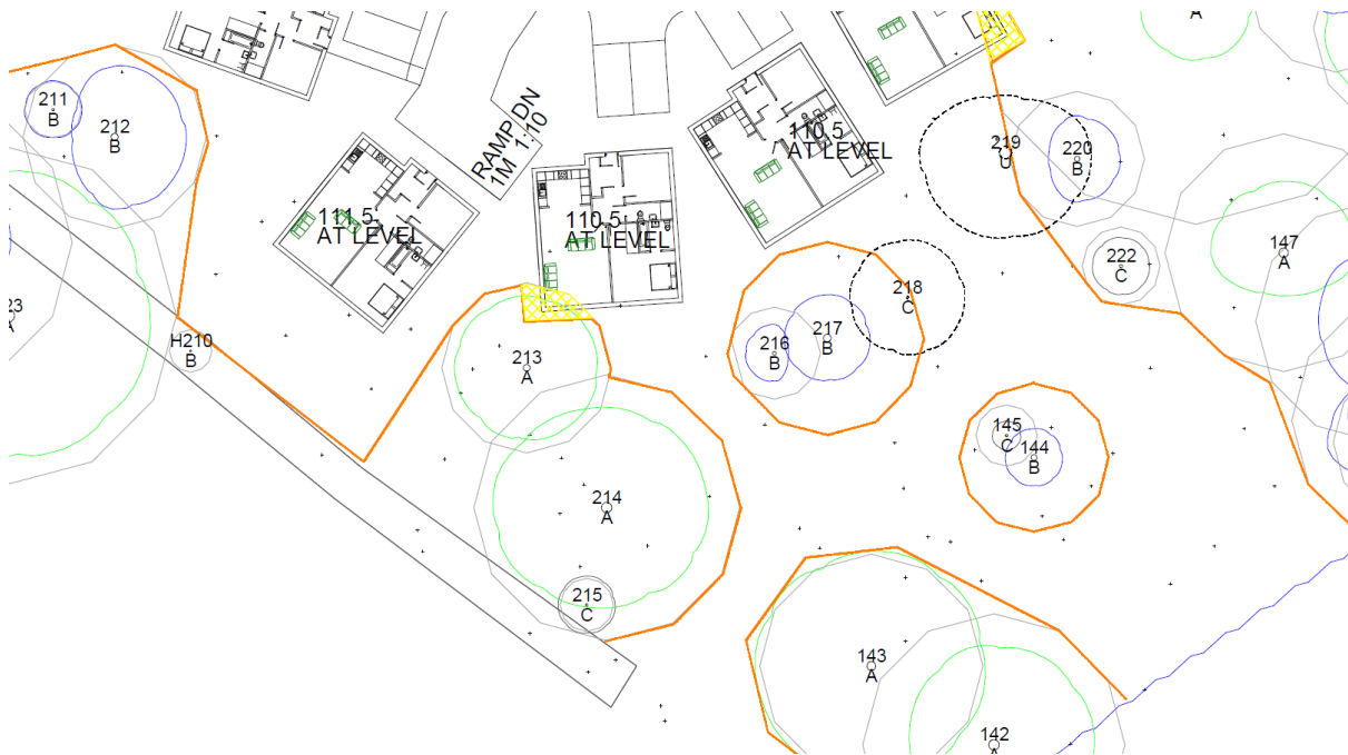
Image 6: T213 & T214 in close proximity to the proposed building. The canopy of T213 will be on the roof and will require annual tree work, or a significant crown reduction on this side - extracted from the applicant's Tree Protection Plan.
