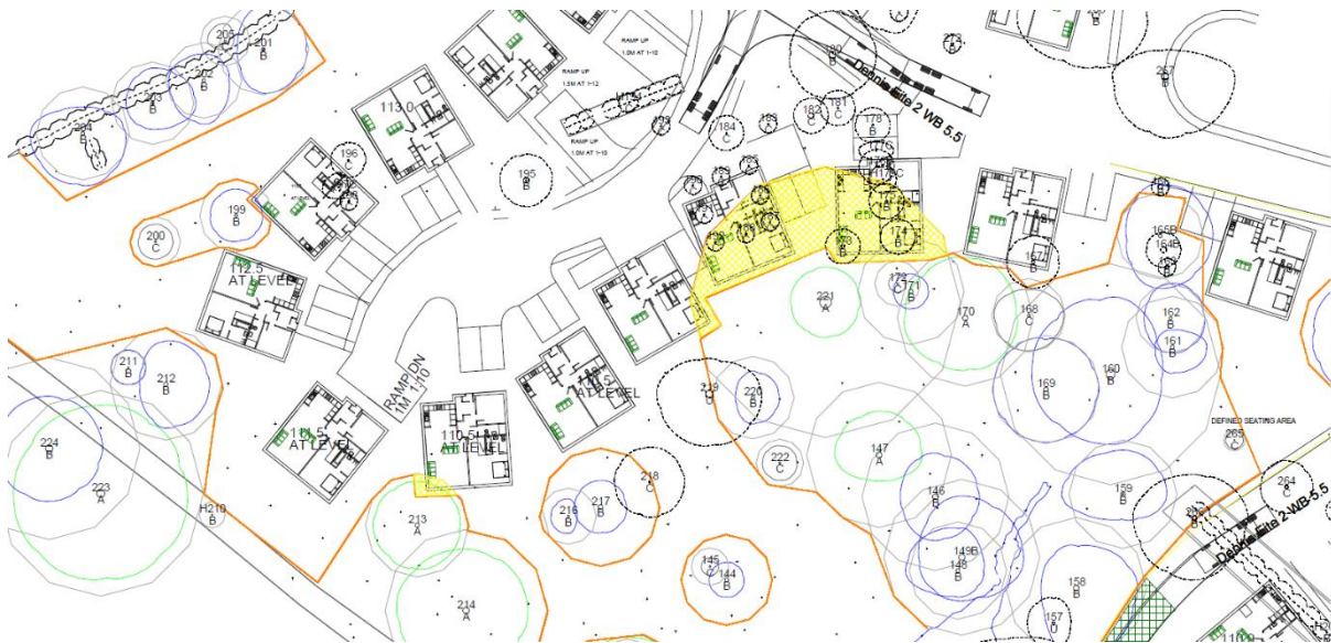
Image 4: Yellow area in middle of image shows amount of construction within the root protection area of T221 and adjacent trees, as well as proximity to buildings post development - extracted from the Tree Protection Plan.
